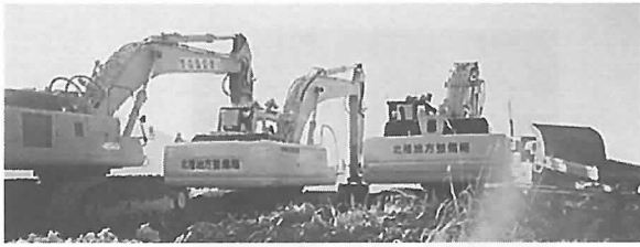
Photograph 28 The radio controlled construction machine that was used the rescue work.
