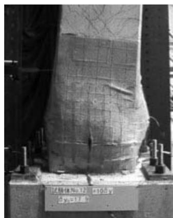
**Fig.12 PET jacket performance after large plastic deformation**
